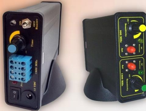
This device is designed for detection and identifying mobile radio transmitters of cellular communications standards (mobile phones and modems of GSM 900, 1800, UMTS), wireless data transmission (WI FI and BLUETOOTH).
